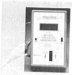
☑ The MX1000 Pressure Generator provides a safe alternative to mercury manometer calibration methods. The MX1000 can simulate either a positive or negative pressure in mmHG.
