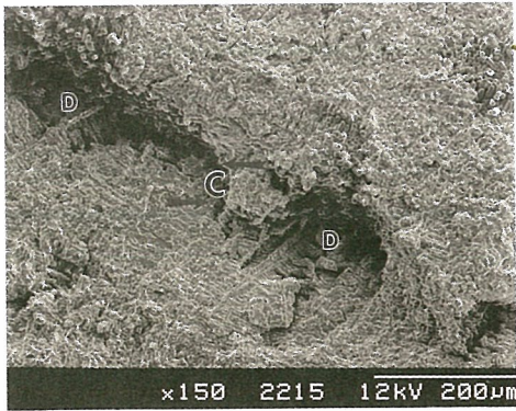
Fig. 8. Crack (C) propagating along the dendritic crystals (D) at the fracture surface.
