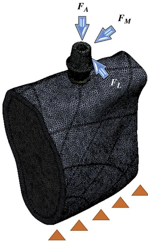
Figure 2 Load and boundary conditions applied to the three-dimensional finite-element method models. The bottom of the model was fixed and the implants were loaded with forces of 17.1 N ( F_L ), 23.4 N ( F_M ), and 114.6 N ( F_A ) in the lingual, mesio-distal, and axial directions, respectively.
