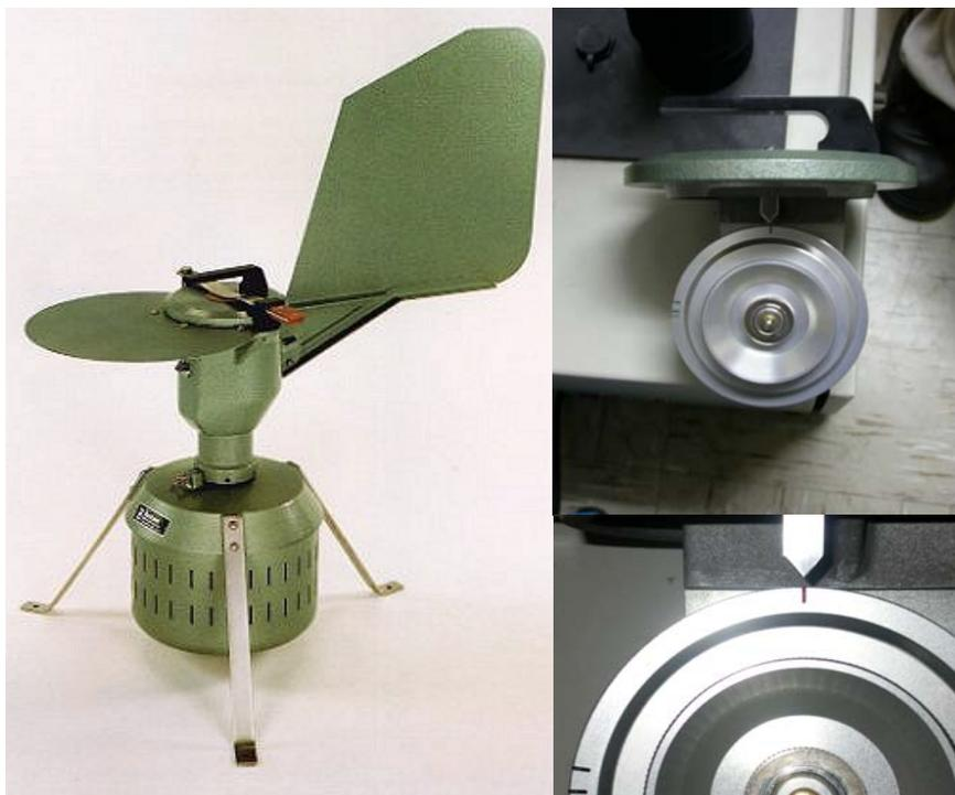
圖二 Burkard Seven-Day Recording Volumetric Spore Trap
