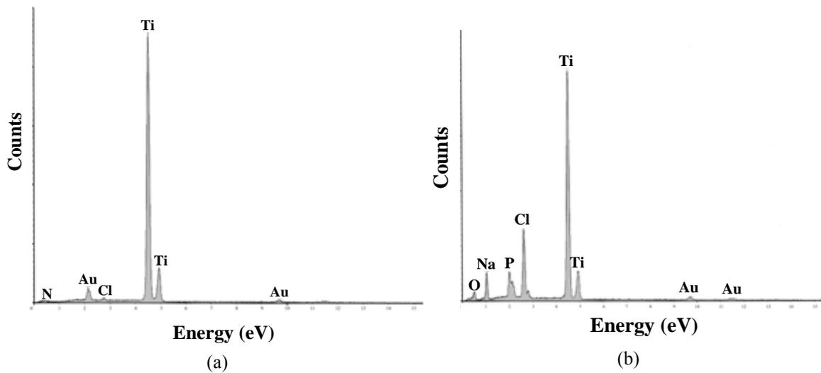
Figure 4 shows energy dispersive spectrometer (EDS) is performed to detect the titanium surface that has undergone various chemical treatments: (a) Ti without surface treatment, (b) glutaraldehyde treated Ti surfaces.
