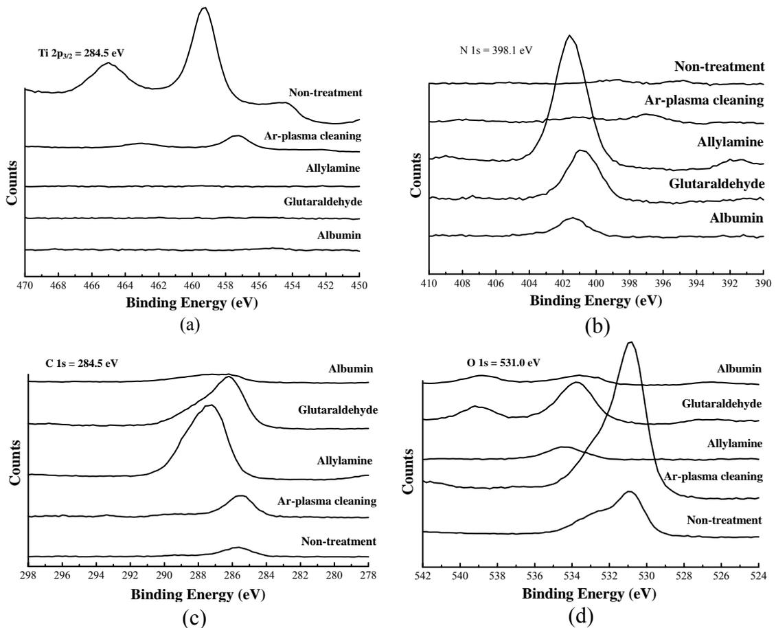
Fig. 5. X-ray photoelectron spectroscopy (XPS) is used to analyze surface deposition changes of Ti surfaces that have undergone various chemical treatments.
